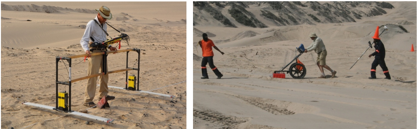
Fig 23: GPR Test Surveying: Medium Frequency (100MHz) and High Frequency (900MHz)
